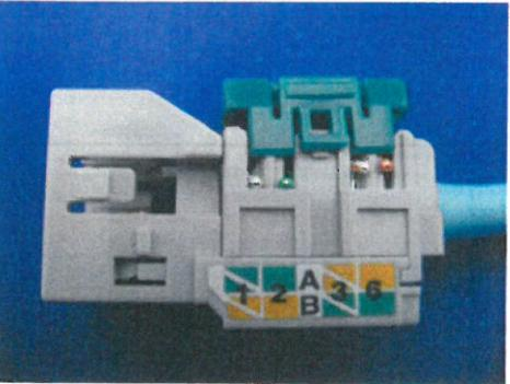
A photograph of a modular jack termination where the wires are crimped onto the contacts. The wires are visible protruding from the side of the connector. The text "17" is written in a box in the bottom right corner.                                                                                       | 17     |
